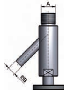
Probierventil test valve
